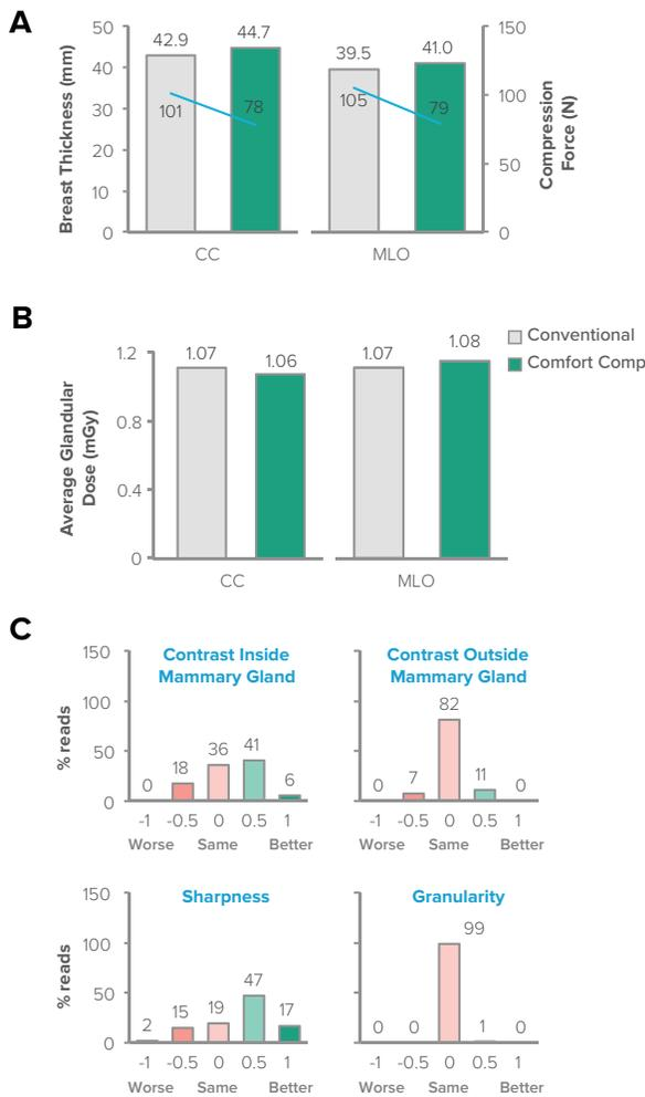
**Figure 3. Comfort Comp compression reduction does not affect breast thickness, average glandular dose, or image quality.** A, Compression force effects on breast thickness. B, Compression mode impact on average glandular dose. C, Image contrast, sharpness, and granularity obtained with conventional and Comfort Comp modes were evaluated by a qualified reader using a 5-point scale.
